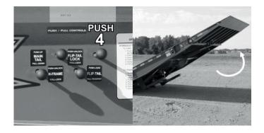
Push the FLIP-TAIL lever to rotate the flip tail into position.
