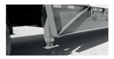
MANUAL JACKS - pull the release pin to let the foot fall. Make sure you stand clear of the parking jack foot.
