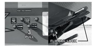
Pull the FLIP-TAIL LOCK lever to engage the flip tail lock.
