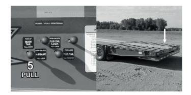
Pull the MAIN TAIL lever to lower the tail to transport position.
