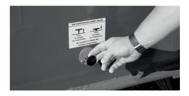
If your trailer has an air suspension, dump the air from the trailer suspension by pulling the Air Suspension Dump Valve control lever. This will provide a lower loading angle.
