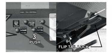
Push the FLIP-TAIL LOCK lever to release the lock on the flip tail section.
