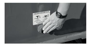
Push the AIR SUSPENSION DUMP VALVE button to raise the suspension for transport.
