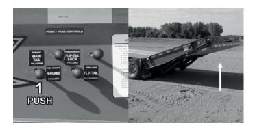
First raise the MAIN TAIL by pushing the corresponding control lever.
