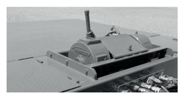
Your trailer may be equipped with an upper deck winch. Please read the instructions that came with the winch for operation.
