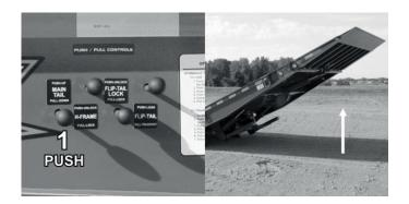
To reposition the tail section for transport, start by pushing the MAIN TAIL control lever to raise the entire tail section.
