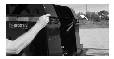
If you need a higher transport height for road clearance, you can use the additional load plate spacers.
