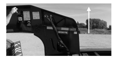
Using the hydraulic control lever, raise the gooseneck until the load plates can be opened.
