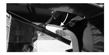
Using the support arm control lever, lower the gooseneck support arm to the tow vehicle. Use enough pressure to support the gooseneck, but not raise it.
