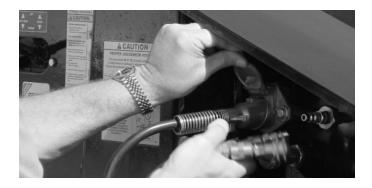
Remove the air and electrical lines from the gooseneck to the trailer bed.
