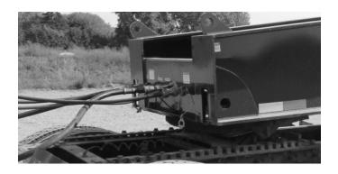
Start the hydraulic system so that oil is flowing to the gooseneck. If your trailer has the pony motor option, start the pony motor according to the instructions on the pony motor decal.
