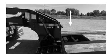
Using the control levers again, lower the gooseneck to the ground. Stand clear of the deck.
