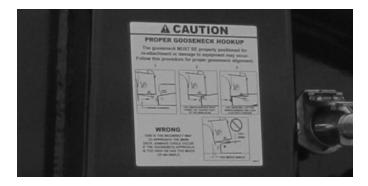
Read the CAUTION decal to make sure the undercarriage is set properly before backing into the main deck or damage may occur.
