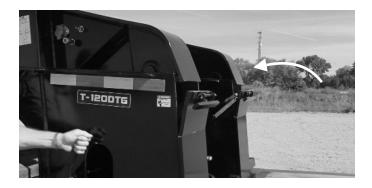
Continue lifting the deck until the support plates can be closed.
