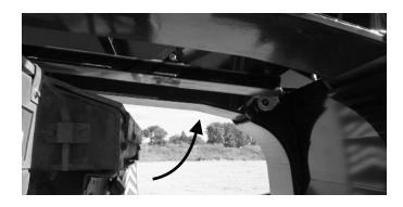
Using the control lever, lift the gooseneck support arm off the truck frame.
