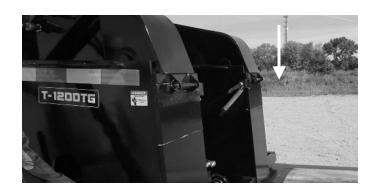
Lower the gooseneck until it rests on the load plates.
