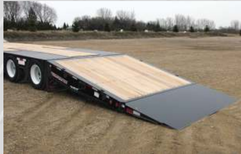
Hydraulic tail creates a low load angle and easy approach. Rear tail section folds under when in transport position.
