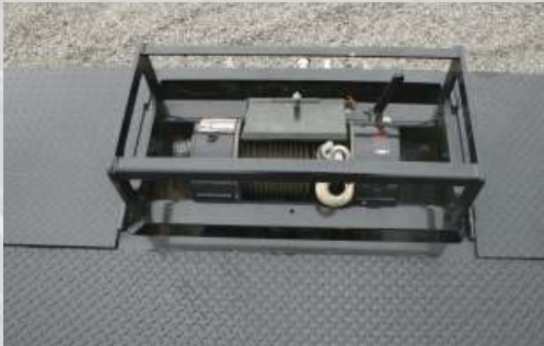
12K hydraulic winch with cable is standard. It is positioned at the front of the 10-foot upper deck of the HT trailer.
