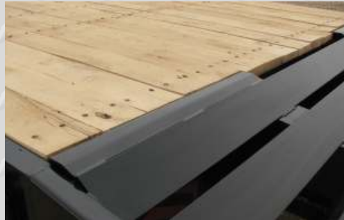
Wood protectors are standard on Towmaster T-series trailers and protect the end of the deck boards.
