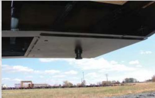
S.A.E. King Pin with smooth approach plate for easy hook-up.
