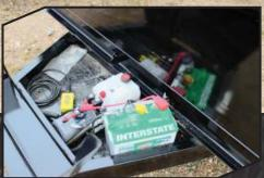
Built-in storage box houses hydraulic system with room for chains, straps or tools.
