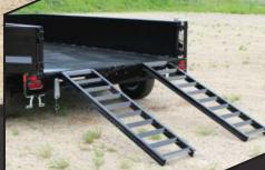
Ladder-style ramps are standard and are stored under the bed.
