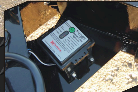
Sealed battery break-away system charges while plugged into the tow vehicle and can be checked at the press of a button.
