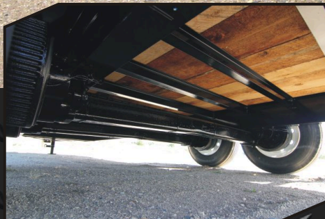
Dexter's heavy-duty 12,000 lb. Torflex rubber-ride axles with oil-bath hubs provide a smooth ride.
