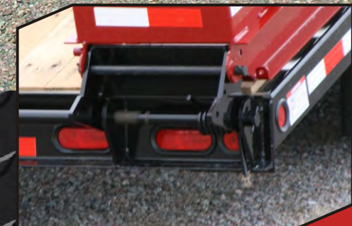
One-way spring-assist ramps and grommet mounted incandescent lights.
