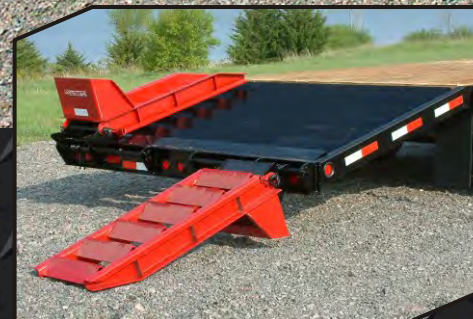
Angle-iron beavertail and ramps provide excellent traction for loading and unloading.
